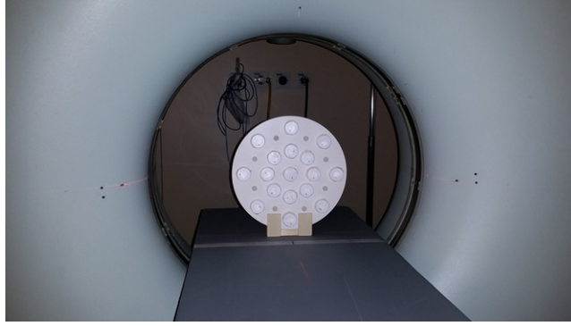
Figure 1. Detail of the phantom used to hold the liquid substances used to verify the calibration.
