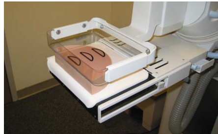
Figure 7. Contrast-detail phantom set-up: 1 foam pad.
