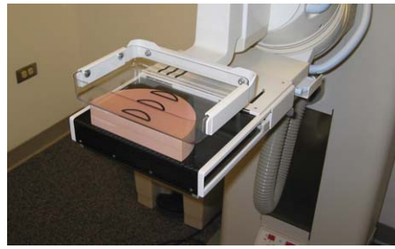
Figure 6. Contrast-detail phantom set-up: no foam pads.
