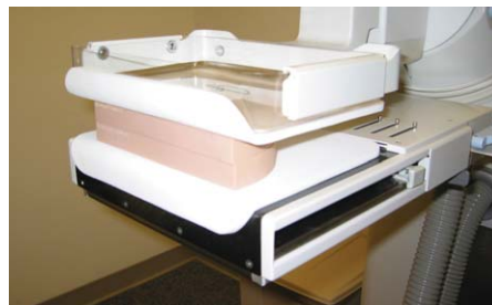
Figure 8. Contrast detail phantom set-up: 2 foam pads.
