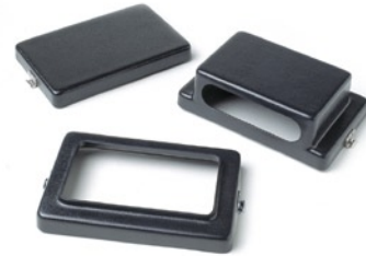
Phantom includes detachable scanning wells and air tight case.
