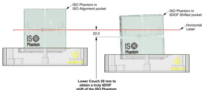
Take a set of images that are to be used by the system to calculate the rotation and translation shifts. Apply the calculated couch shifts and take another set of images, which now should produce shifts that are close to zero. The difference between zero and the actual values for each individual shift should be within the setup tolerances.
