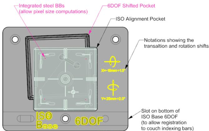
Align the ISO phantom to the imaging system that is to be used to acquire the image reference set. To do this, place the ISO base on the couch of the imaging system (CT) and register it to an indexing bar. Use a high quality spirit level and level it. Place the ISO Phantom in the ISO alignment pocket.
