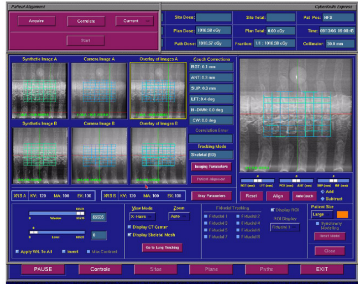
Using Xsight Spine Tracking System for initial phantom alignment
