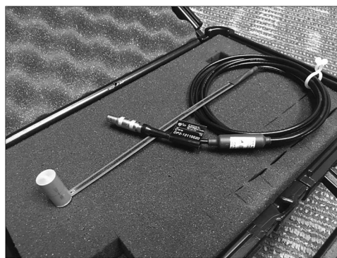
Figure 2. The CTD P -2 solid-state detector. The solid-state detector employed in this study was customized from a commercially available CTD P .
