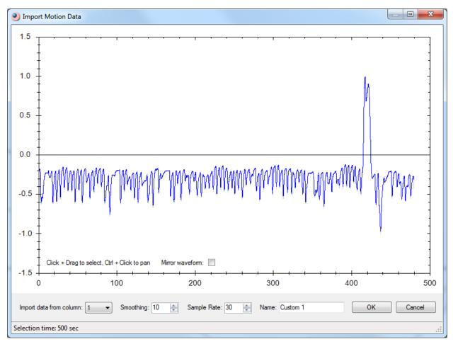
Because the software allows different waveforms to run for each of the phantom's axes, the user has to import the data from each column that contains tumor positions in a 3D space separately in order to be able to select the appropriate waveform for each of the phantom's motions.
