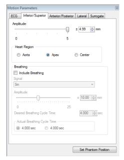
The Linear Inferior/Superior tab allows also the user account for the movement of the heart due to the breathing.
