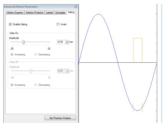
When the Invert box is checked the effects of "Gate On" are reversed.
