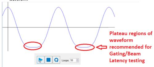
Send the target to the amplitude corresponding to the plateau regions from Start Position slider bar/entry box (see below). Before doing this make the amplitude of Inferior/Superior zero.
