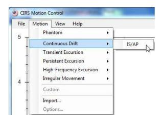
□ *IS/AP* sets both *IS* and *AP* directions amplitudes of the centroid of the prostate, which are needed for the software to calculate the correct linear motion of the phantom's actuator.
