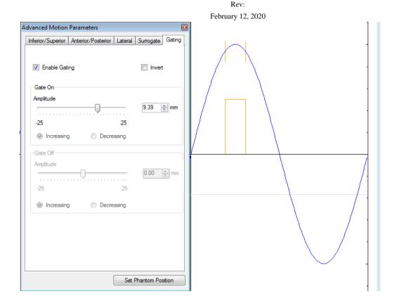
The gating signal has a value of +5 V when the Inferior-Superior amplitude is equal or smaller than the "Gate On" value for negative amplitudes. When the Inferior-Superior amplitude is greater than the "Gate On" value the gating signal has a value of 0 V.
