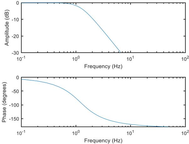
Fig. 4. Properties of implemented low-pass filter
