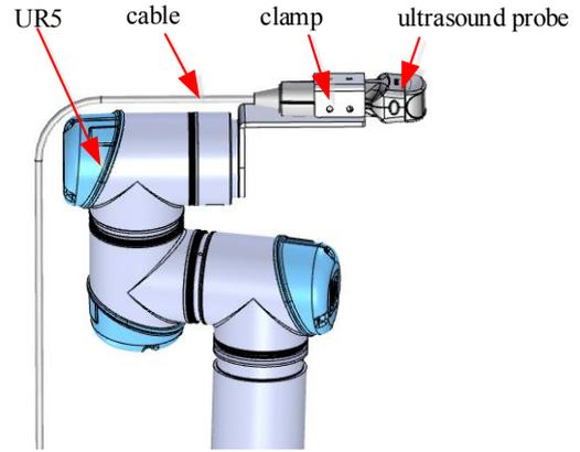
Fig. 2. Clamp is designed to hold probe .
