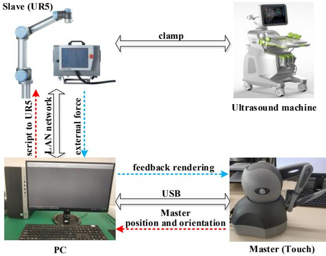
Fig. 1. Configuration and connection of the system and flow of information
