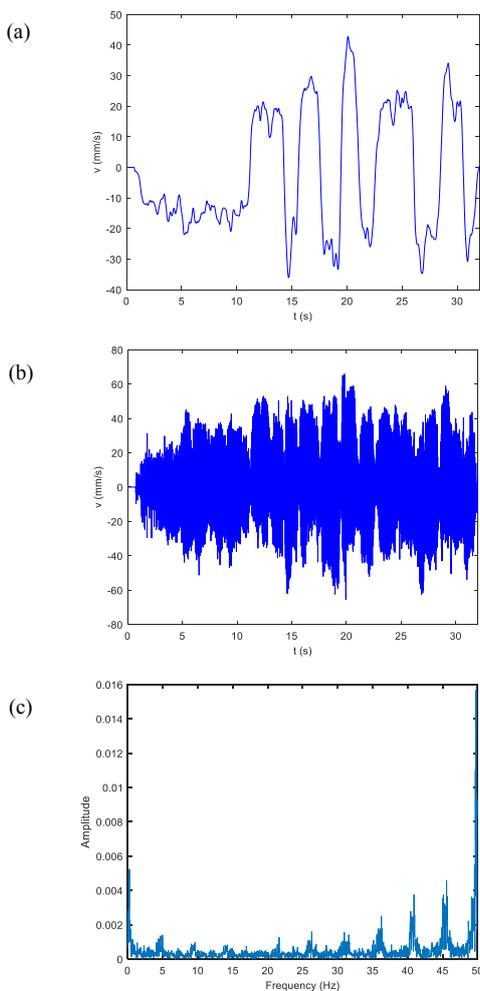
Fig. 6. (a) The filtered speed of the Touch in the y-axis of the slave base coordinate (b) UR5 Tcp actual speed in z axis, (c) Spectrum of (b)
