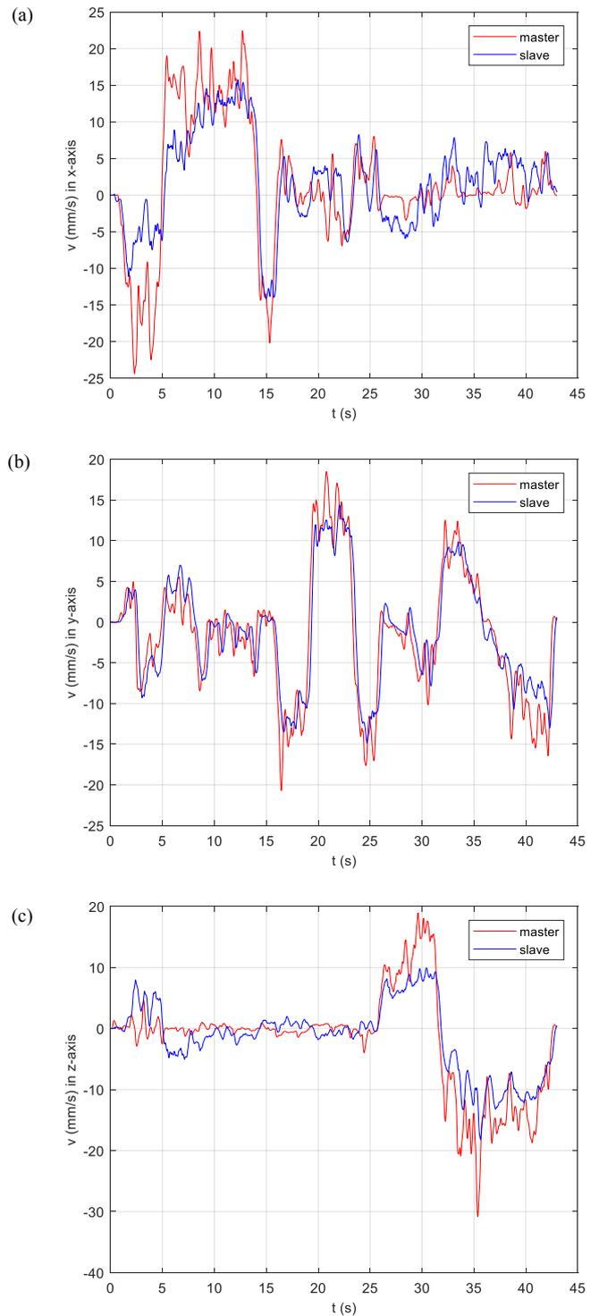
Fig. 7. Comparison of master and slave speed in slave base coordinate: (a) in slave x-axis, (b) in slave y-axis and (c) in slave z-axis
