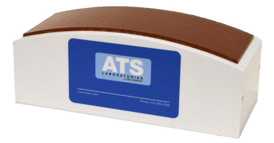
The ATS UC-551M, a modified version of the ATS Model 551 Small Parts Phantom, is designed for use with GE's Invenia ABUS scanner. The scan surface has a 17.5-inch radius of curvature, which matches the shape of the Invenia ABUS scan head.
