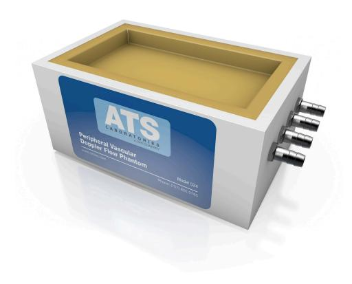
The Models 524 and 525 tissue mimicking Doppler flow phantoms contain four flow channels simulating superficial vasculature. The simulated vessels are located 15 mm below the scan surface. Built-in scanning wells are provided to permit the use of water or a low viscosity gel as acoustic coupling agents.
