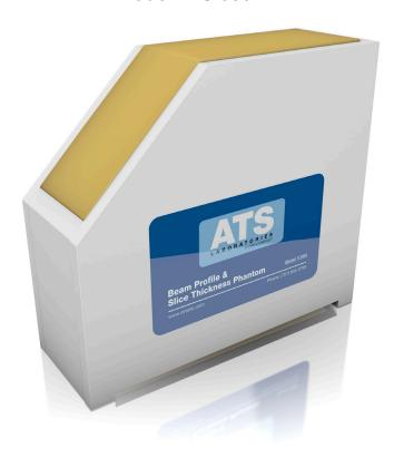
The model 538NH can measure the beam profile and slice thickness of ultrasound imaging systems by evaluating the appearance of a thin plane of echogenic material against an anechoic background.
