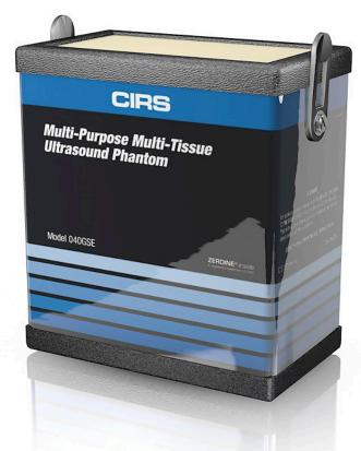
The CIRS Model 040GSE Multi-Purpose, Multi-Tissue Ultrasound Phantom is the most complete solution available for performance and quality assurance testing. Its dual frequency design and detachable water wells allows testing of most transducer shapes – including curvilinear and endocavity – and frequencies. It is also the only QA phantom on the market that provides both elasticity targets and all the standard B-mode imaging test objects.
