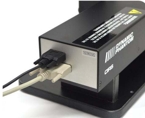
**2.** Plug the Cable DB9 m/m which leads from gating device to back of actuator.
