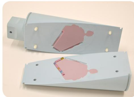
3. The Dynamic Cardiac Phantom Target Detection Rod 008C-01 is supplied with replaceable targets that simulate different iodine and calcification concentrations in the arteries.
