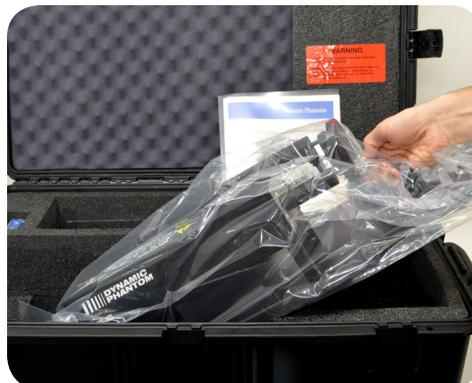
7. Pull base and the actuator assembly from case.
