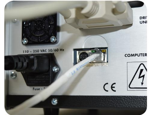
**3.** Attach ethernet cable to back of controller.
