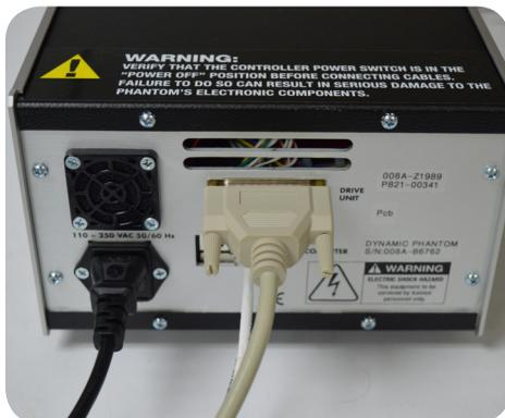
**4.** Plug power cord into the back of controller. Plug other end of power cord into the wall outlet.
