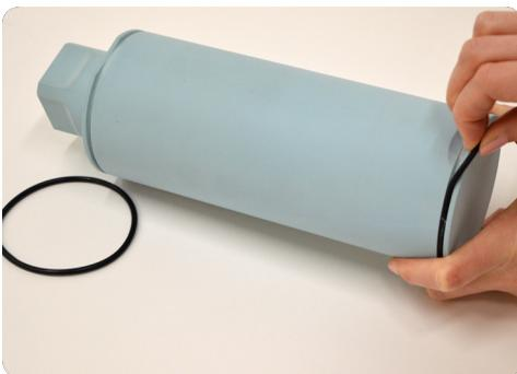
2. To access these pockets remove both O-rings and carefully pull the two halves apart
