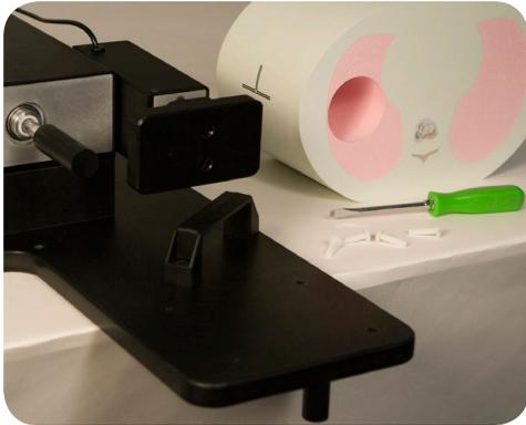
**1.** Place base plate with actuator assembly on table. Carefully move base plate to overhang table. This allows access to holes for attaching phantom body.
