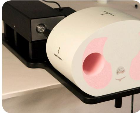
**2.** Position phantom body on base plate as shown. To ensure proper alignment for model 008C, the phantom face with the CIRS label should be facing away from the actuator.
