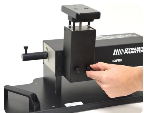
**9.** Move 3rd axis device to vertical position by loosening screws and repositioning as shown.
