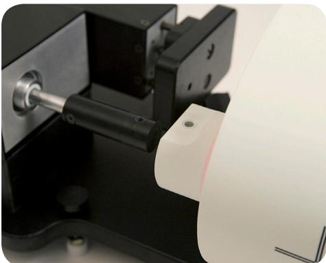
**4.** Insert rod thru hole in phantom body. Ensure that screw hole on rod is aligned with screw hole on actuator rod.
