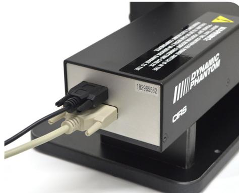
5. Plug the Cable DB9 m/m which leads from 3rd axis gating device to back of actuator.
