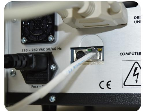
6. Attach Ethernet cable to back of controller.
