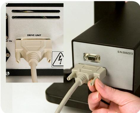
4. Plug the Cable DB25 m/m to back of controller and to back of actuator.
