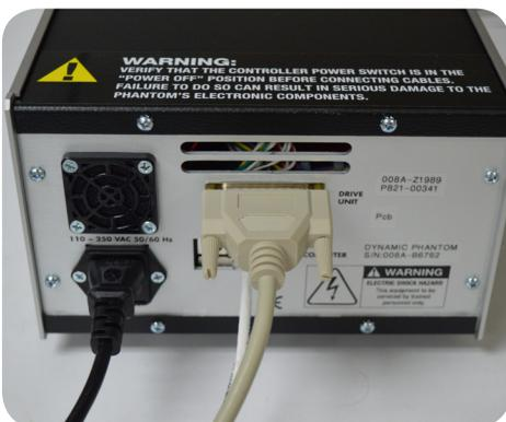
7. Plug power cord into the back of controller. Plug other end of power cord into the wall outlet.
