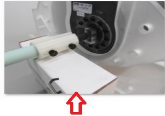
Support the fiberglass shaft assembly while connecting it to the MRI Moving Rod
