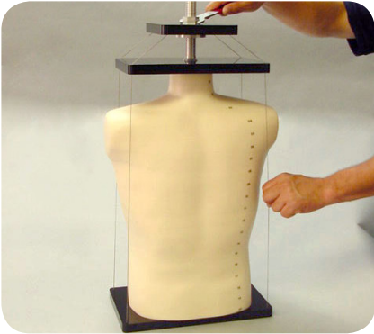
8. Optimal tension is reached when the strings give off a high-pitched tone when plucked with the finger.
