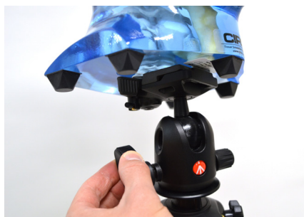
To adjust the positioning of the head, turn lever until head is placed in desired position.
