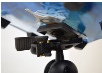
Place quick connect on tripod, make sure it is secure prior to release
