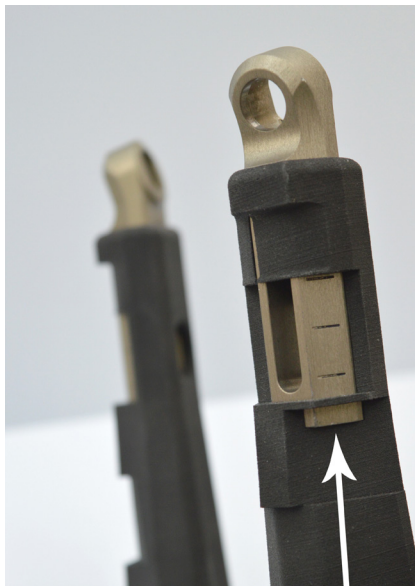
1. Adapter for integrating STEEV and Leksell® Coordinate Frame G.
