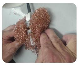
Put the RF filter and cable connectors between two copper mushes and slide them into the waveguide.
