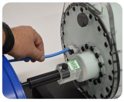
Insert ion chamber into each cavity hole. (Kidney)
