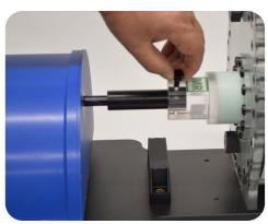
**2.** Place rod into phantom body and screw the rod and actuator together.
