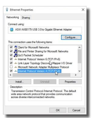
7. In the internet Protocol Version 4 (TCP/IPv4) properties window, change from default "Obtain an IP address automatically" to "Use the following IP address:" Enter "192.168.0.101" as the IP address and "255.255.255.000" as the Subnet mask. Note: If an IP address conflict occurs because IP address 192.168.0.101 is already assigned to another Net work Adapter, the user can try any other IP address between 192.168.0.102 and 192.168.0.249.
