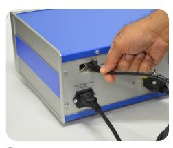
Attach ethernet cable to back of controller.
