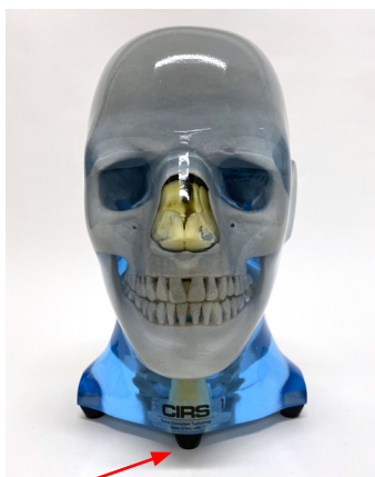
Positioning feet are used to position the phantom on flat surfaces. Note: the positioning feet are not removable.
