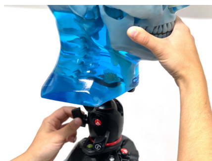
To adjust the positioning of the head, turn lever until head is placed in desired position.
