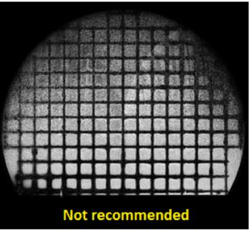
When selecting the FOV, make sure it does not end close to a plane that can be constructed through grid intersections, which are supposed to have the same X or Y or Z coordinate. If the FOV ends close to such a plane, the grid intersections from that plane will be rejected (see below) due to lack of signal from all 6 sides of the intersections. Make sure, based on the slice thickness, the FOV extends more than 5mm on each side of the intersections from the plane.
