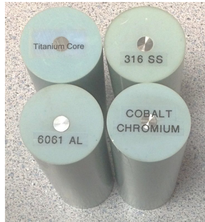
FIG. 2. Custom metal sample plugs designed from plastic-water inserts for the CIRS Model 062 RED phantom. CT number values from these samples were used as data points to characterize the extended CT scale HU to RED conversion curve in the extended range.
