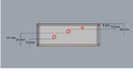
Features one 1/8" vessel with 1/16" wall thickness; two 3/16" vessels with 1/16" wall thickness
