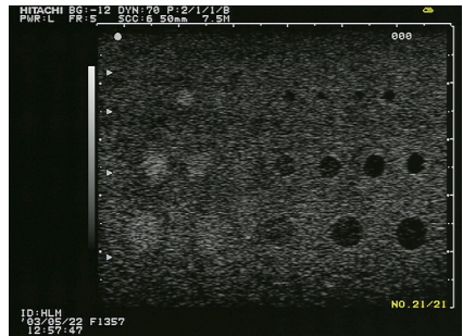
Masses are angled for continuous assessment over a range of depth
