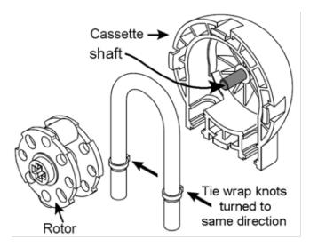
Place tubing into the guide of the cassette, tie wrap knots facing cassette. This will be a tight fit and will NOT snap into place.
