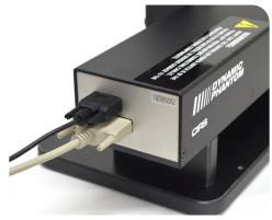
Plug the Cable DB9 m/m which leads from gating device to back of actuator.
