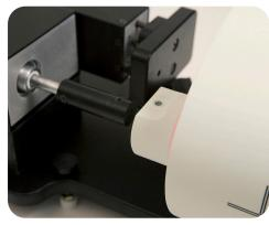
Insert rod thru hole in phantom body.
