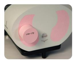
Repeat step 6 with rod extended out. Check gap on the motor box side of body as well. Adjust phantom body to achieve best fit. Finish tightening the screws on underside of phantom.
