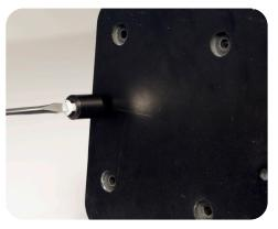
Prior to attaching phantom body, carefully lay base plate with actuator in its side. Attach solid black post to underside of base plate as shown.
