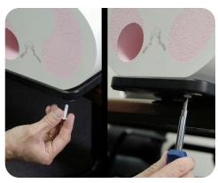
3. Place one screw through bottom of base plate and screw into phantom. Continue until all screws are in place. Snug but do not tighten screws to allow minor alignment adjustments in steps 6 and 7.
