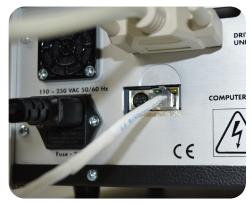
3 Attach ethernet cable to back of controller.
