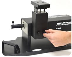
Move 3rd axis device to vertical position by loosening screws and repositioning as shown.
