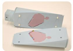
The Dynamic Cardiac Phantom Target Detection Rod 008C-01 is supplied with replaceable targets that simulate different iodine and calcification concentrations in the arteries.
