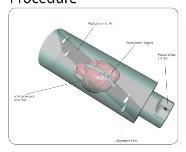
The dynamic cardiac phantom target detection rod is split at a 13 degree angle along the left coronary artery of the embedded heart. The rod is held together via two O-rings at either end of the rod and 4 alignment pins between the two halves. Inner pockets are milled along the edge of the heart to mimic the coronary arteries.
