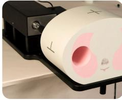
Position phantom body on base plate as shown. To ensure proper alignment for model 008C, the phantom face with the CIRS label should be facing away from the actuator.
