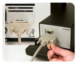
Plug the Cable DB25 m/m to back of controller and to back of actuator.
