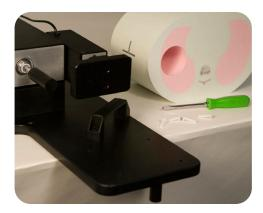
Place base plate with actuator assembly on table. Carefully move base plate to overhang table. This allows access to holes for attaching phantom body.
