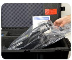
Pull base and the actuator assembly from case.
