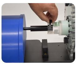
**2.** Place rod into phantom body and screw the rod and actuator together.
