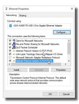
In the internet Protocol Version 4 (TCP/IPv4) properties window, change from default "Obtain an IP address automatically" to "Use the following IP address:" Enter "192.168.0.101" as the IP address and "255.255.255.000" as the Subnet mask. Note: If an IP address conflict occurs because IP address 192.168.0.101 is already assigned to another Net work Adapter, the user can try any other IP address between 192.168.0.102 and 192.168.0.249.
