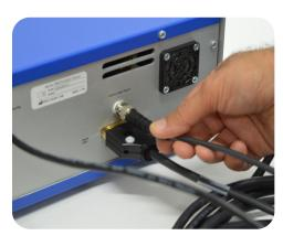
Plug beam latency (BNC) cable into the back of the controller. To perform beam latency, connect the other end of the BNC cable to the Beam-on Beam-off output signal of the MRI-LINAC
