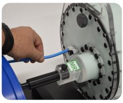
Insert ion chamber into each cavity hole. (Kidney)
