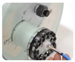
3. Insert ion chamber into each cavity hole. (Moving target)
