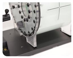
Place phantom body on base plate into the 4 slots as shown in image above.
