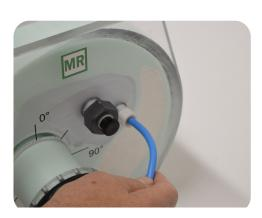
Insert ion chamber into each cavity hole. (Liver)
