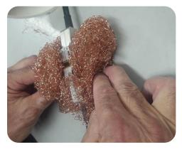
Put the RF filter and cable connectors between two copper mushes and slide them into the waveguide.
