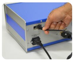
Attach ethernet cable to back of controller.
