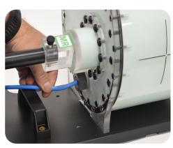
**6** Insert ion chamber into each cavity hole. (Spine)
