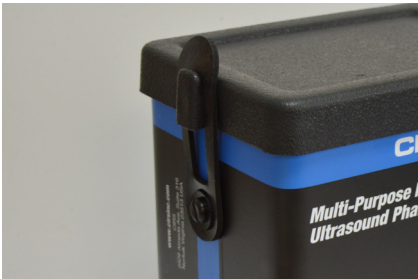
Attach cover with latches
