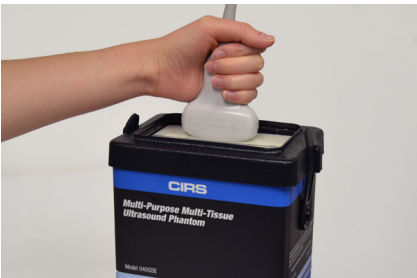
Water well for coupling curved probes
