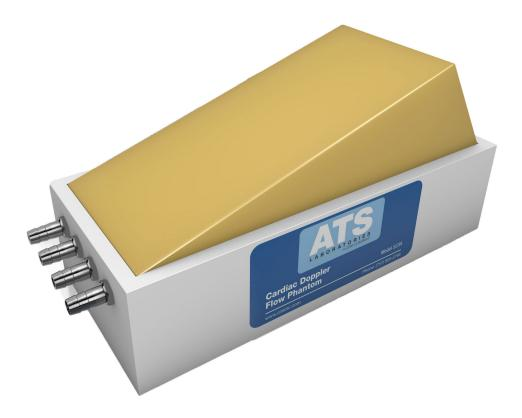
The ATS 523A rubber based tissue mimicking Doppler flow phantoms contain four flow channels of various diameters (normally 2, 4, 6, and 8mm diameter) simulating the deep vasculature of the cardiac and abdominal vessels.
