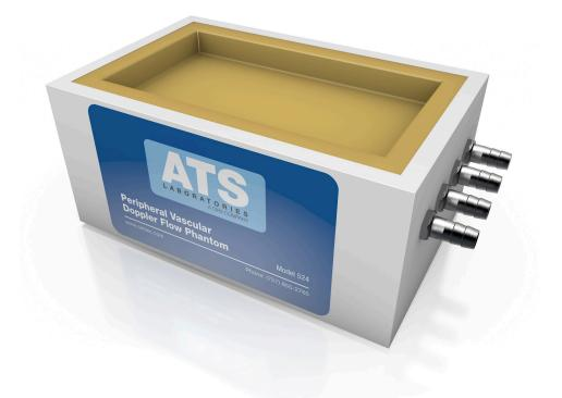
The ATS Model 524 tissue mimicking Doppler flow phantom contains four flow channels simulating superficial vasculature. The simulated vessels are located 15 mm below the scan surface. Built-in scanning wells are provided to permit the use of water or a low viscosity gel as acoustic coupling agents.
