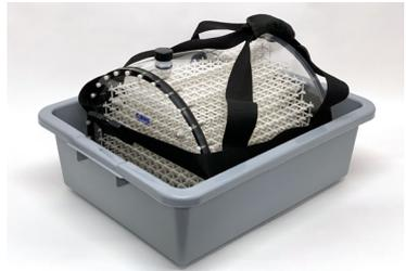
After filling with water, position the phantom in the plastic tray and let sit for approximately 1 hour. Inspect for wet spots. **DO NOT LEAVE PHANTOM UNATTENDED.**
