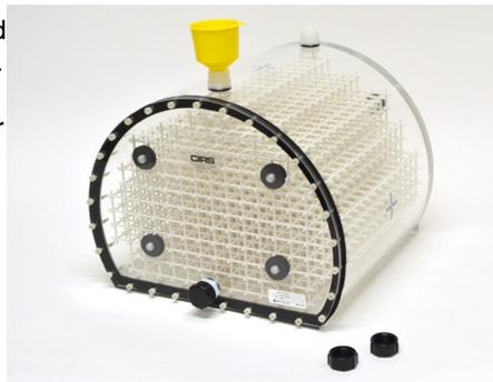
1. Ensure front plate of the housing is secured. The gasket for the front plate should have light, even pressure on the front plate.
