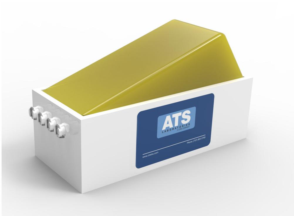
The ATS 523A rubber based tissue mimicking Doppler flow phantoms contain four flow channels of various diameters (normally 2, 4, 6, and 8mm diameter) simulating the deep vasculature of the cardiac and abdominal vessels.
