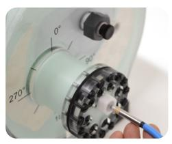
Insert ion chamber into each cavity hole. (Moving target)
