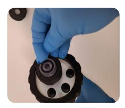
3. Remove the sealing O-ring (a recess in the target threaded part makes this easy to accomplish), check for leakage and wipe off the excess filling solution around the filling hole with a wet towel and then with a dry
