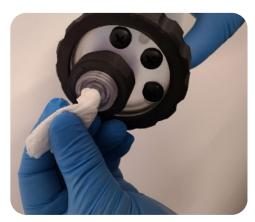
4. Optional: to prevent the filling liquid from flowing into the ion chamber cavity, plug in a rolled piece of paper towel.
