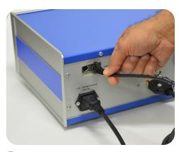
Attach ethernet cable to back of controller.
