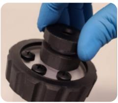
7. Put back the sealing O-ring and secure it in place with the sealing nut.
