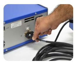
Plug the Cable DB26 m/m to back of controller and to back of actuator.
