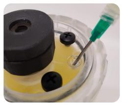
Open one of the filling ports/holes using a Philips screwdriver (it is recommended that the middle filling hole is opened; see above). Purge the air bubble using the provided solution, syringe, and needle. Seal back the rod, check for leakage and wipe off the excess filling solution around the filling hole with a wet towel and then with a dry one.
