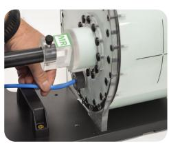
Insert ion chamber into each cavity hole. (Spine)
