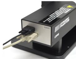
**5.** Plug the Cable DB9 m/m which leads from 3rd axis gating device to back of actuator.
