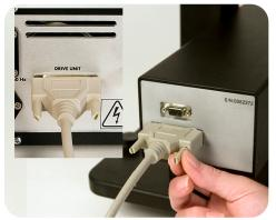
4. Plug the Cable DB25 m/m to back of controller and to back of actuator.
