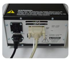
7. Plug power cord into the back of controller. Plug other end of power cord into the wall outlet.
