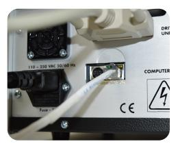
6. Attach Ethernet cable to back of controller.
