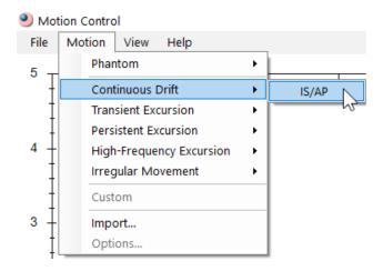
• *IS/AP* sets both *IS* and *AP* directions amplitudes of the centroid of the prostate, which are needed for the software to calculate the correct linear motion of the phantom's actuator.
