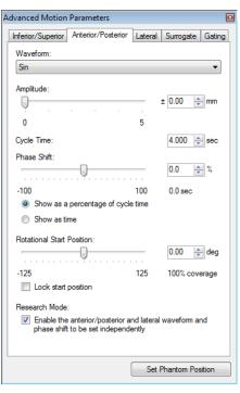
The Surrogate tab allows you to adjust the amplitude, cycle time and phase shift of the surrogate axis (not applicable for model 008Z).
